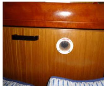
*An additional fire port added such that extinguisher spray could gain access to the top of the engine*
