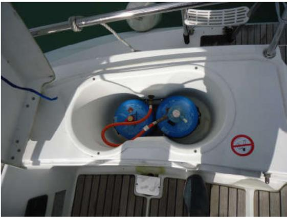
*Gas locker at helm with bottom gas escape hose to external hull outlet”.*
