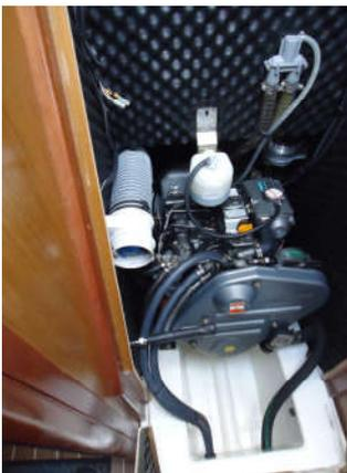
*Engine compartment with inadequate manufacturers installed fire port. Refer to the mallet handle (bottom left) that is projecting through the fire extinguisher port into the engine compartment. It is unlikely that an extinguisher using that port would be able to spray adequate powder onto the engine.*
