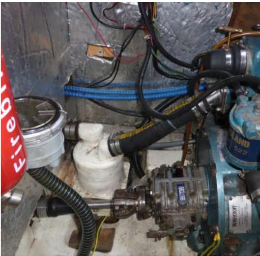
In order to remove the cockpit floor I had to disconnect the steering cable from inside the steering pedestal, remove the pedestal and the 2 legs either side. On the starboard side, the leg houses the Morse controls which operate the gearbox and engine throttle. Both of these were removed at the engine end and the leg lifted out as a complete unit
