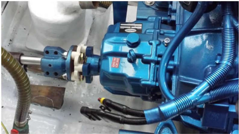
It was now a case of replacing all the old water and fuel hoses with new ones, properly routed around the engine bay, and fitting the new panel. The pre-wired wiring looms made this very easy, just connect the 2 multi-plugs together.
