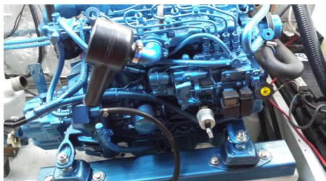
The whole lot was then bolted down again, having put a bed of Sikaflex under the new box sections. The engine was then bolted to this and re-alligned with the propeller shaft having now fitted a new R&D coupling
